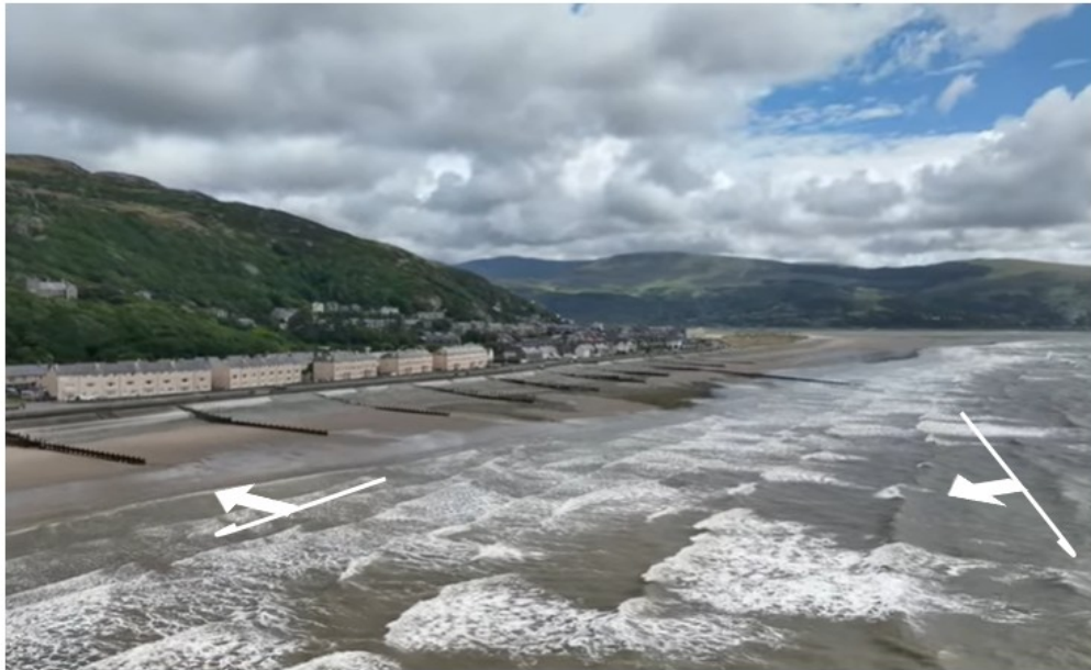
Figure 14. Waves approaching Barmouth from the south west are slowed as they enter the shallow coastal water and swing around to approach the beach more directly towards the sea wall.
